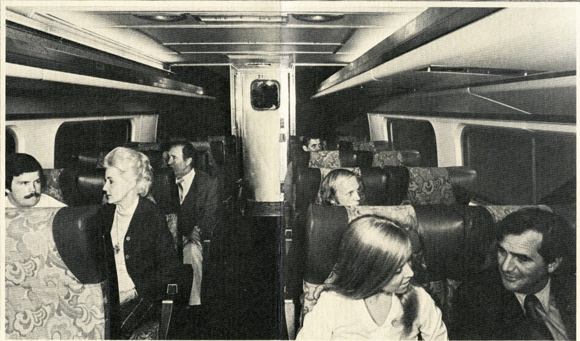
Spacious, color-coordinated interiors—combined with thermal and acoustical insulation and an air and coil spring suspension system—offer maximum passenger comfort at high operating speeds. Each Amcoach and Amcafe food service car features electric heating and air conditioning.
